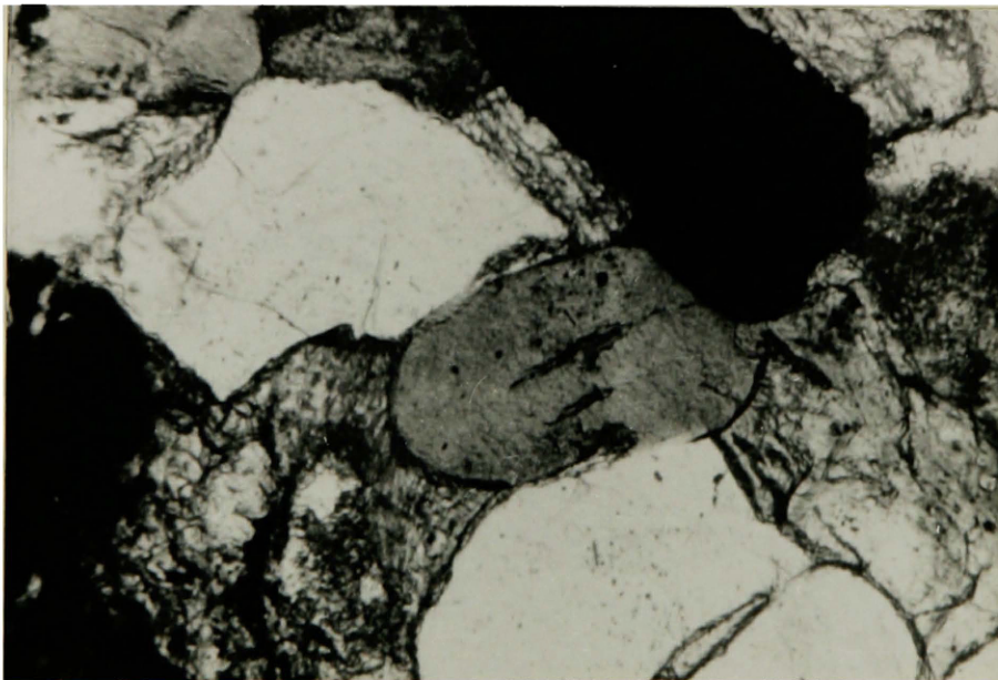
Figure 15. Yellowish green rounded glauconite in the Swift sandstone. Sample from Bradman Railroad section at 56 feet from base. X 80.
