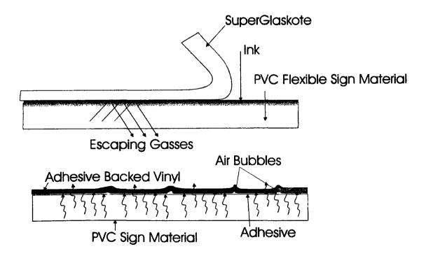
The flexible sign material when it is new is less porous than when old. The very small holes in the material surface expand with age. As the material ages, the holes expand and a gas is released from within the material to the surface of the material (called plasitizer migration). This gas moves to the sign surface and causes small bubbles in the applied graphics. Eventually this gas will eat or cause problems with the adhesive that holds the graphic to the flexible sign material.
