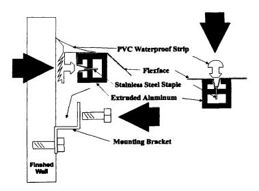
Figure 7: Poly's awning extrusions and frame joints
