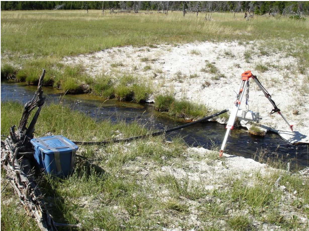
Figure 17. FloDar set up at Rabbit Creek 5 gallon storage tote for scale. Photo by Jacob Mohrmann, 2006
