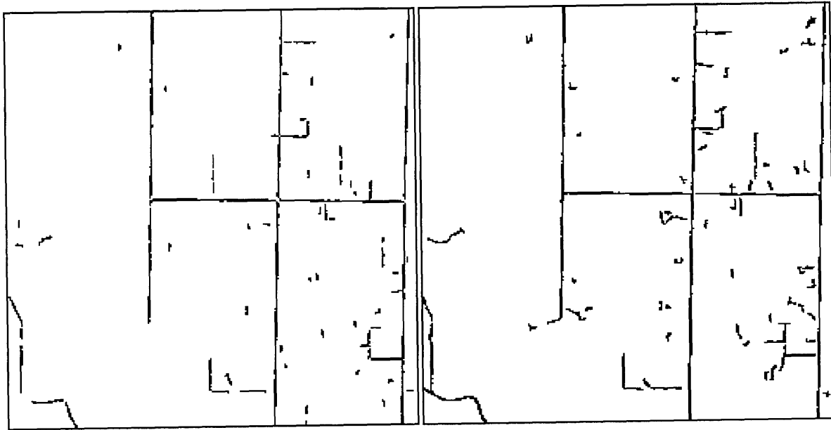
Figure 6: Typical ANN results on road image using 9 \times 9 foveal representation.
