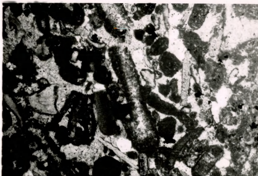
Carbonate Sand Rock Type Algal plates, lumps, pellets, intraclasts and fossil fragments in sparry matrix.
