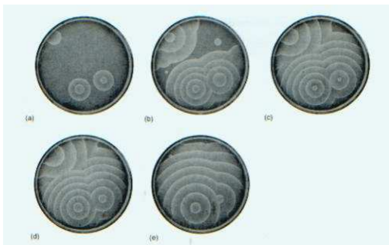
Figure 1: Target Patterns in a Thin-layer of BZ Reagent in a 9-cm Diameter Petri Dish
