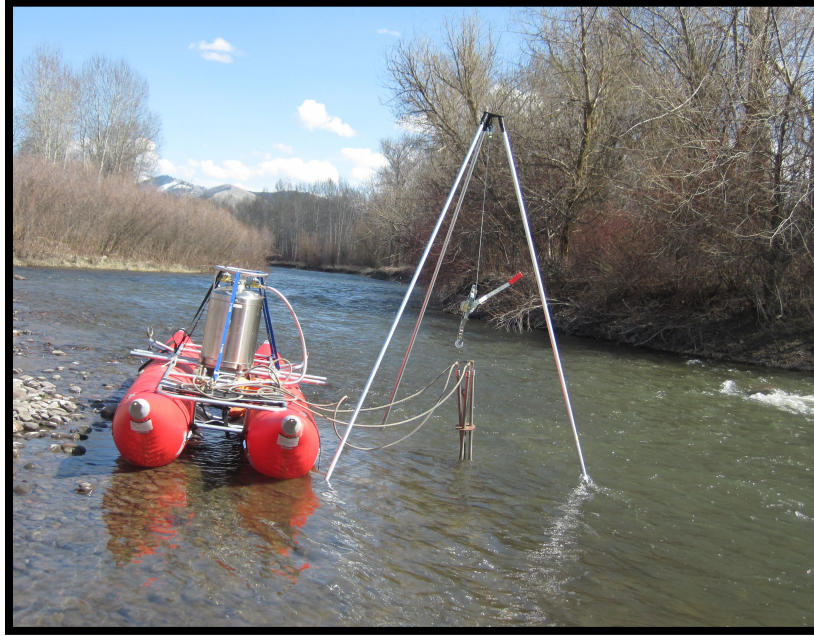
Figure 6. Photo of freeze core equipment in place. To collect the sample, pressurized nitrogen from the nitrogen tank was inserted into the injection rods. The nitrogen cooled the water surrounding the poles, freezing the sample to the poles. The tripod and come-along, hanging over the nitrogen injection rods, were then used to remove the sample from the bed.
