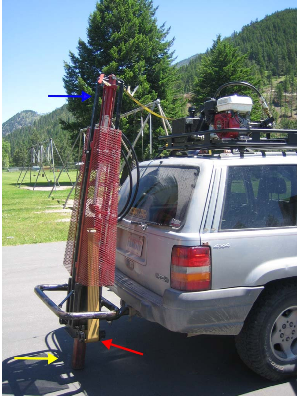
Figure 5: Bison Industries elastic wave generator. This accelerated weight drop system works by dropping a steel beam (yellow arrow) into the ground. The beam is lifted using a hydraulic ram (blue arrow) and is accelerated into the ground using a large elastic band (red arrow). This source is capable of generating a large amount of seismic energy.
