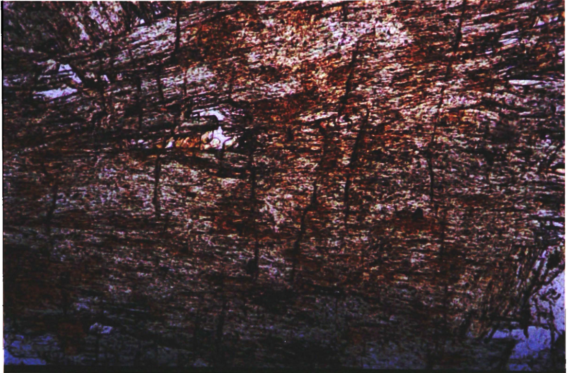
Figure 23. Biotite alteration of hornblende (1mm FOV).
