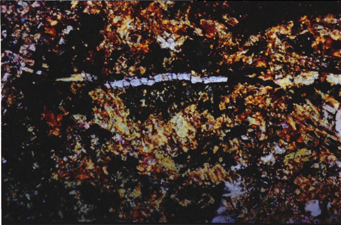
Figure 19. Quartz-epidote veinlet with local extreme alteration (3.5mm FOV).
