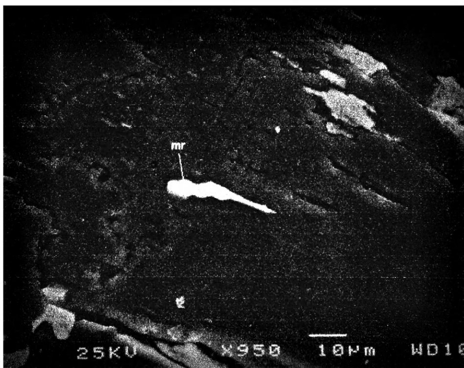
Figure 22. SEM BEI showing mertieite (mr) grain in hydrothermal quartz.
