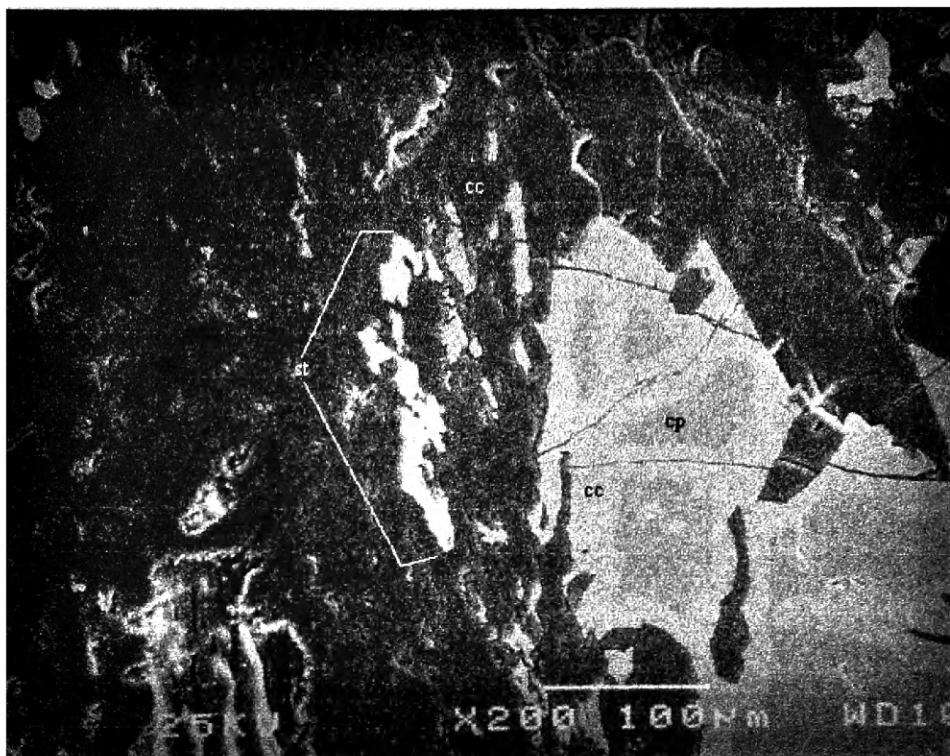
Figure 21. SEM BEI showing long vein-like stibiopalladinite (st) grain in mass of very fine grained hydrosilicate minerals (chlorite and or epidote). This grain conglomerate can also be seen in Figure 11. Note chalcopyrite (cp) rimmed by secondary chalcocite (cc).
