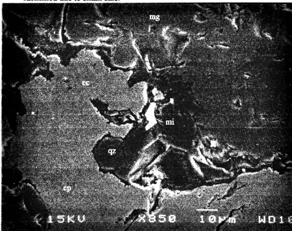
Figure 26. SEM BEI showing a michnerite (mi) grain in quartz (?) (qz) between chalcocite (cc) and magnetite (?) (Mg). Note small amount of remaining chalcopyrite (cp)
