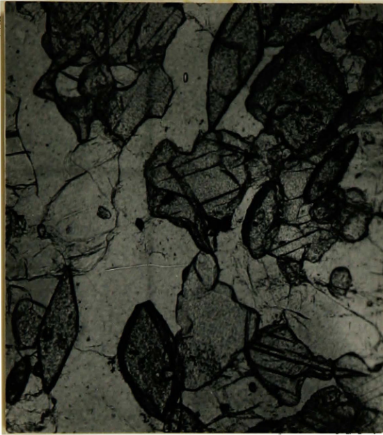
Figure 16. Pyroxene-quartz-plagioclase rock with well formed sphenes prisms. Loc. 9-9-3. Plane light x 58.
