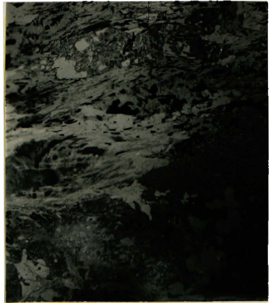
Figure 19. Chloritized and sericitized gneiss. Loc. 9-2-1. Plane light x 17.
