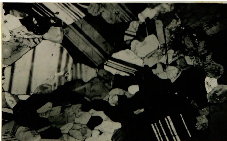
Figure 12. Typical texture of the massive andesinite. Crossed nicols, x 17.
