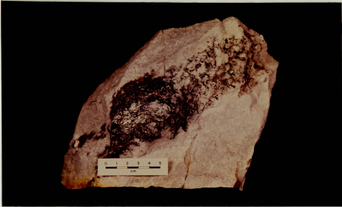
Figure 19: Textural Type V. Sulfide pod in calcite and barite. Sulfides include sphalerite and jamesonite. Note yellow smithsonite in upper-right corner. Hoodoo Mine.
