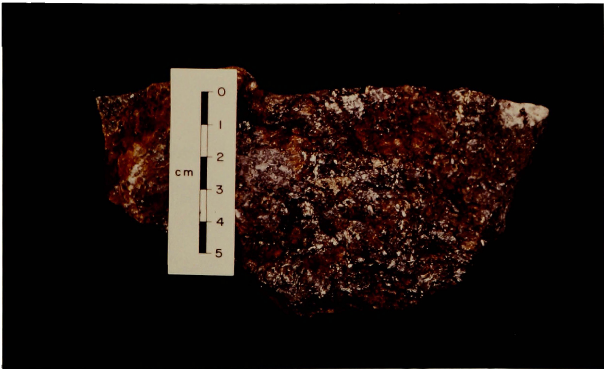
Figure 23: Textural Type VII. Jamesonite on fracture in rhyolite. Livingston Mine.
