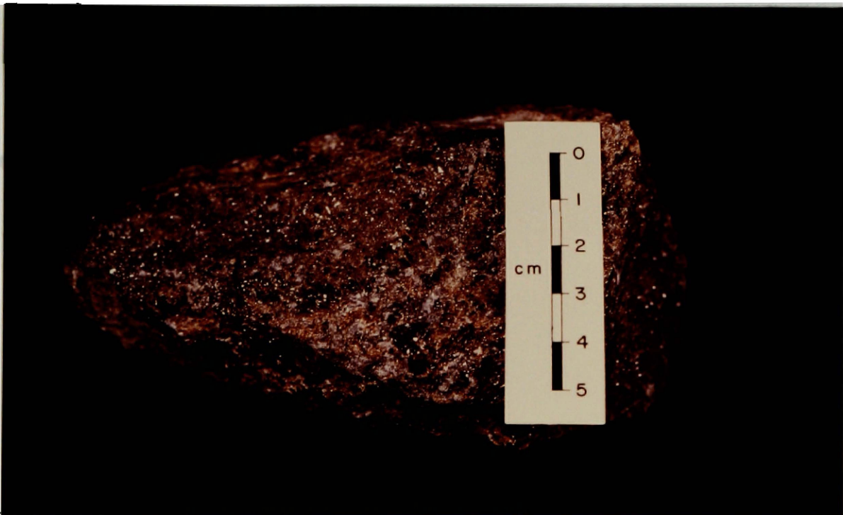
Figure 15: Textural Type IIIa. Massive sphalerite with minor carbonaceous wall-rock fragments. From cross-cutting vein structure. Hoodoo Mine.
