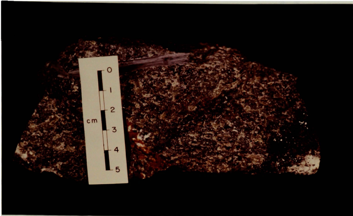
Figure 22: Textural Type VII. Disseminated pyrite and sphalerite in rhyolite. Livingston Mine.
