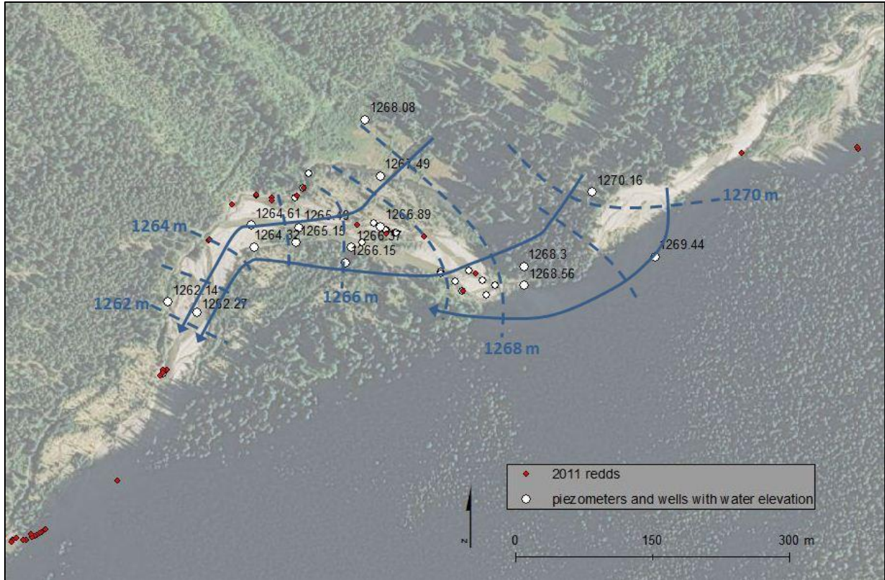
Figure 22. Ole Creek water table contour map encompassing OLE mc and OLE sc on 9/11/11. Dashed blue lines are water table contours with blue elevation numerical labels. Solid blue lines are inferred subsurface flow direction lines. (NAIP (2011) photos)
