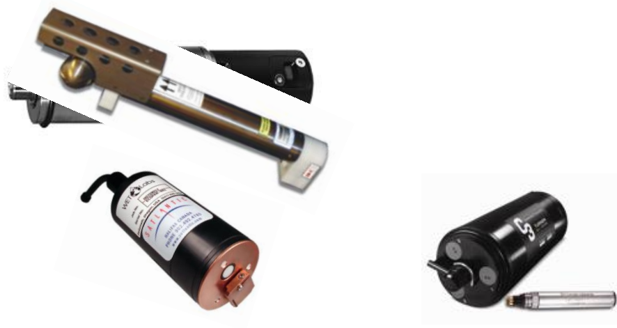
Figure 2.4. Sensors deployed with the SAMI or on the profiler: Aanderaa oxygen sensor (on SAMI) (top left), Microcat CTD sensor (on SAMI) (top right), Satlantic PAR sensor (on profiler) (bottom left), and WETLabs Chl- a sensor (on profiler) (bottom right).
