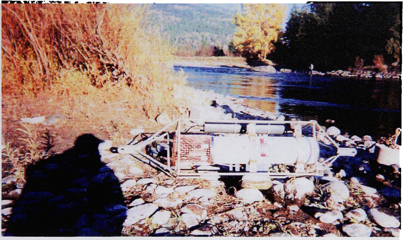
Figure 3.14. SAMI-pH in the protective cage, ready for deployment
