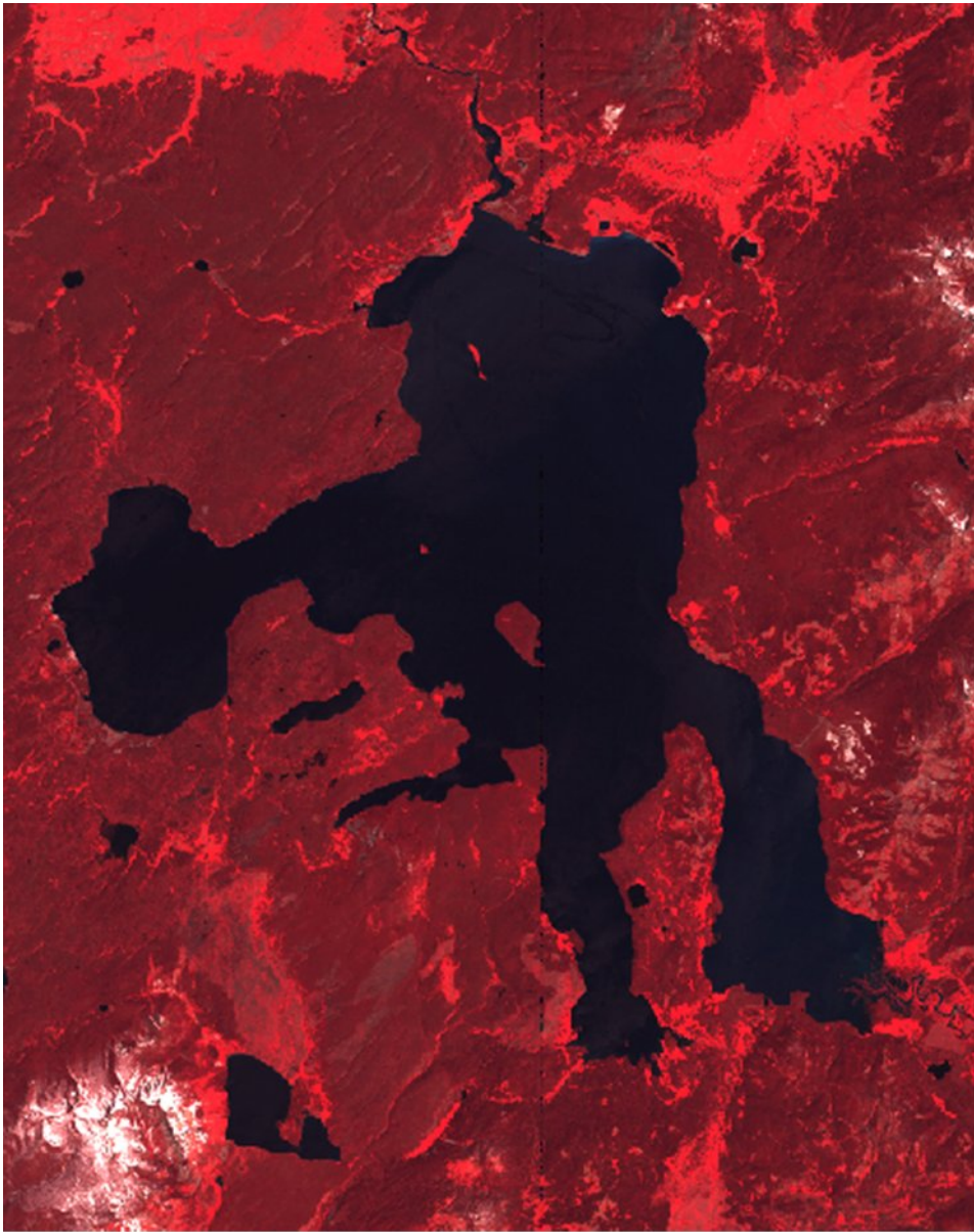
Figure 5.8 False color composite of the Yellowstone Lake region. Lighter shades of red are indicative of riparian/grassland vegetative zones while the darker shades reflect closed forest canopy.
