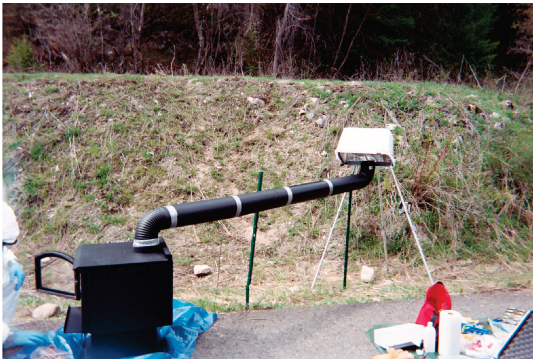
FIGURE 2. Woodstove combustion study setup.
