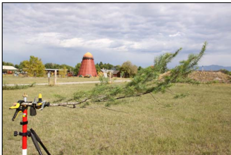
Figure 1. Douglas-fir specimen mounted on tripod in the 0^\circ position.
