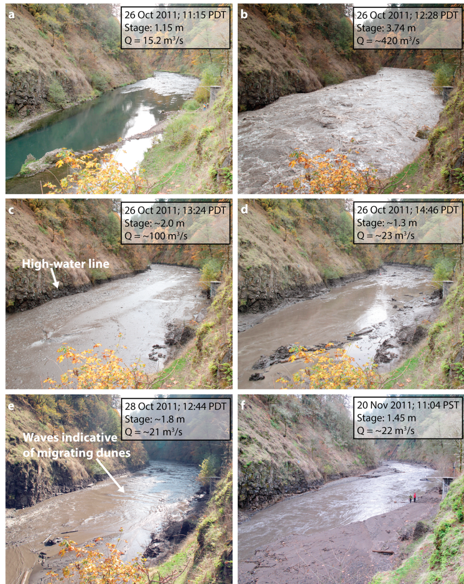
Figure 5. White Salmon River at USGS gauge site 2.3 km downstream of dam site, looking downstream: (a) 53 min before breaching; (b) 20 min after breaching, at discharge peak; (c) 76 min after breaching, at peak sediment concentration, with high water line evident; (d) ~2.5 h after breaching, discharge has returned to background and sediment concentration is falling; (e) 2 days after breaching, when channel has aggraded and migrating dunes indicate substantial sandy bed-material transport; and (f) 25 days after breaching, showing bar emergence.
