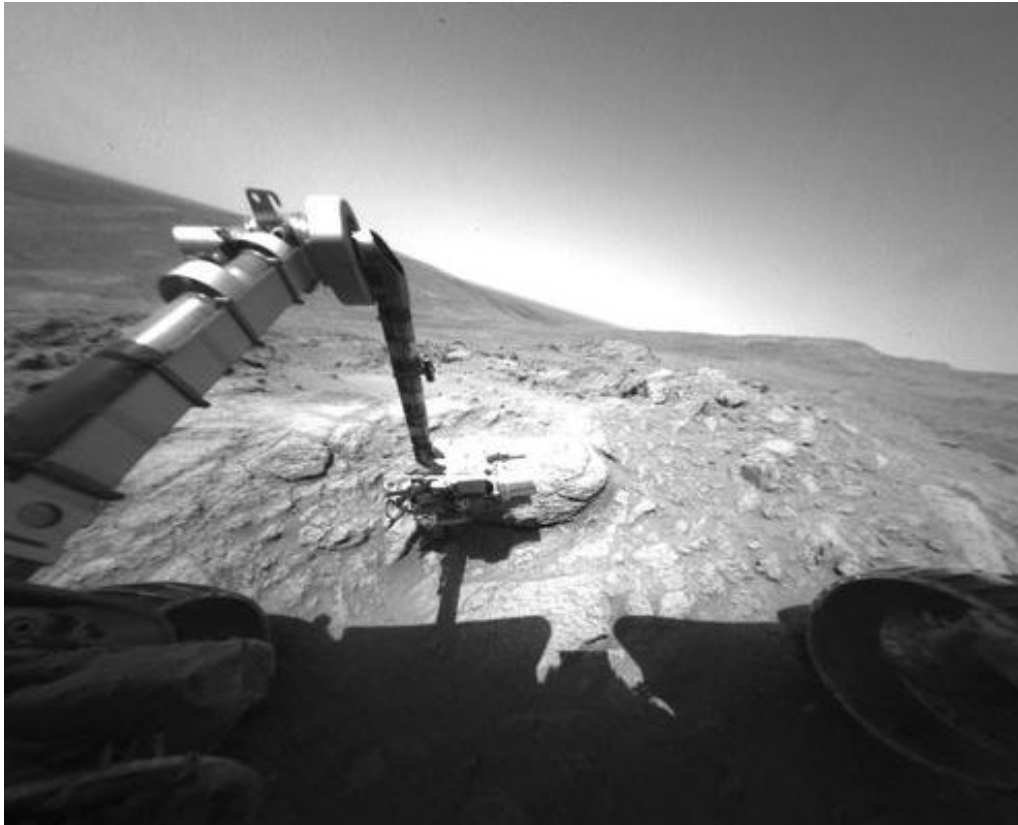
Figure 9 The Mars rover Spirit moves its robot arm over a Martian stone in order to take a series of pictures with its microscope camera. http://marsrovers.jpl.nasa.gov/gallery/press/spirit
