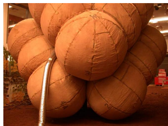
Figure 5 Left: Wind tunnel test of the MER landing module parachute. http://www.nasa.gov/centers/ames/images/content/79641main_picture_2.jpg Right: MER landing module airbags. http://photojournal.jpl.nasa.gov/jpegMod/PIA04999_modest.jpg
