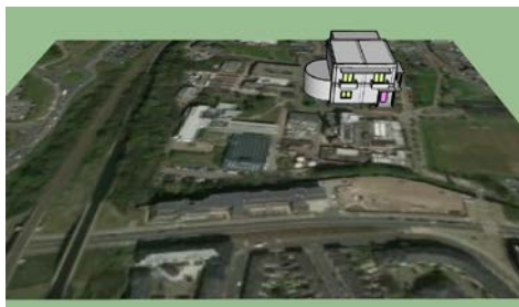
Figure 5. Ten IFC buildings superimposed onto the satellite image of the University of Birmingham, UK campus.
