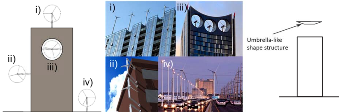
Figure 2. a,b) WT and buildings: i) on rooftop, ii) on façade, iii) integrated, iv) in vicinity; c) flow enhancer [20].
