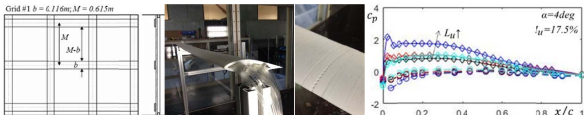
Figure 1. a) Schematic of passive grid used to generate inflow turbulence; b), c) experimental setup at the university of Liège; d) preliminary results showing the effect of LS.
