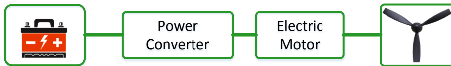
Figure 2. Block diagram of all electric propulsion system
