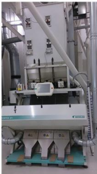
Figure 2. Sortex Z+ Optical Sorter
