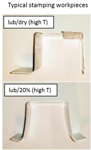
Fig. 7. Assessment of L_{left}/L_{right} and L_t of top-hat parts forming using WC: C coated tools at BHF=5kN, T=20°C, 430°C.
