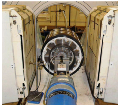
Figure 3: The experimental rotating drum in the field of view of the Birmingham ADAC Forte gamma camera.
