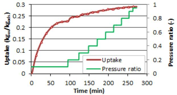
Fig. 4 DVS test results at 36°C for AQSOA-Z02
