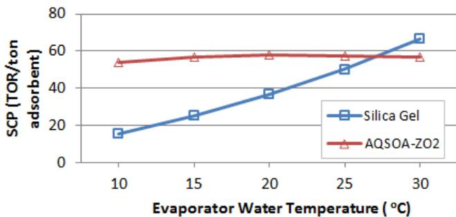
Fig. 13 SCP at 85°C hot water temperature.
