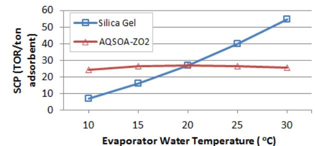
Fig. 11 SCP at 75°C hot water temperature.
