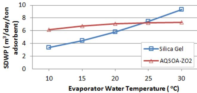
Fig. 12 SDWP at 85°C hot water temperature.
