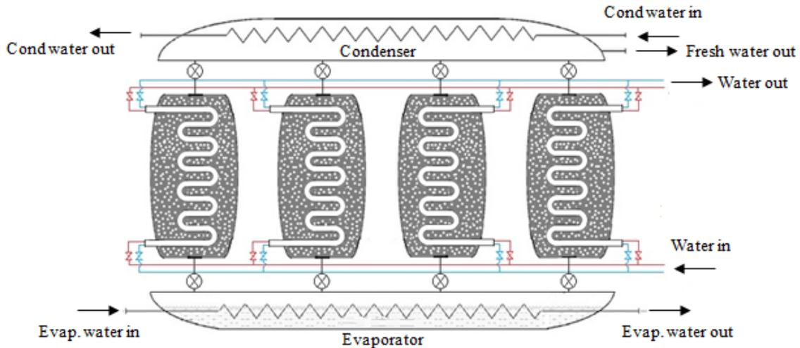
Fig. 1 Schematic diagram of the adsorption system
