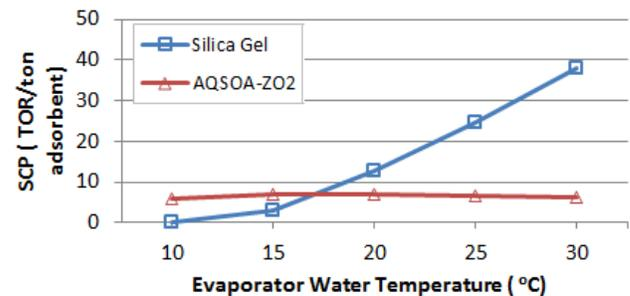
Fig. 9 SCP at 65°C hot water temperature.
