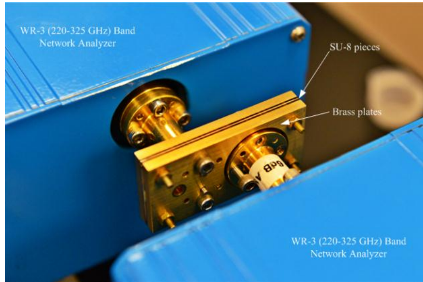
Figure 6: A photograph shows the device WR-3 waveguide under test with the Network Analyser.
