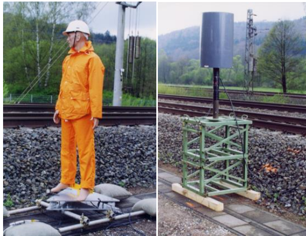
Figure 10 The dummy and cylinder used in the RAPIDE trials (33)
