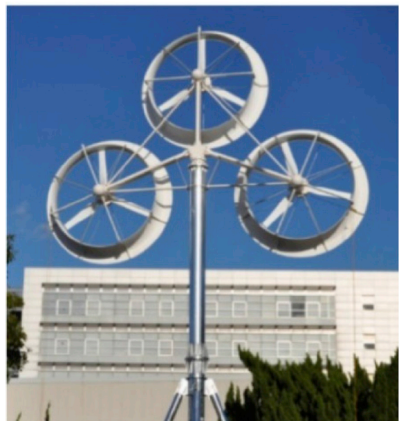
Fig. 9. 10 kW multi-rotor DAWT system installed in Japan. Courtesy of Kyushu University and Riamwind Corporation.
