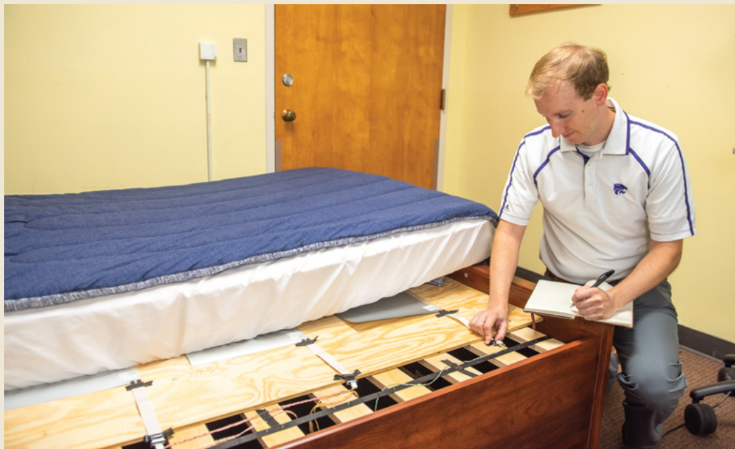
Charles Carlson, teaching assistant professor of electrical and computer engineering, sets up sensors under the mattress of the smart bed.
