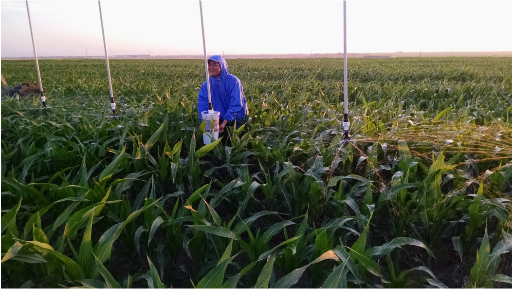
Figure 2. Measuring spray nozzle flow rate using a Spot-on device to compare with design flow rates at the Kansas State University Southwest Research-Extension Center, near Garden City, KS.
