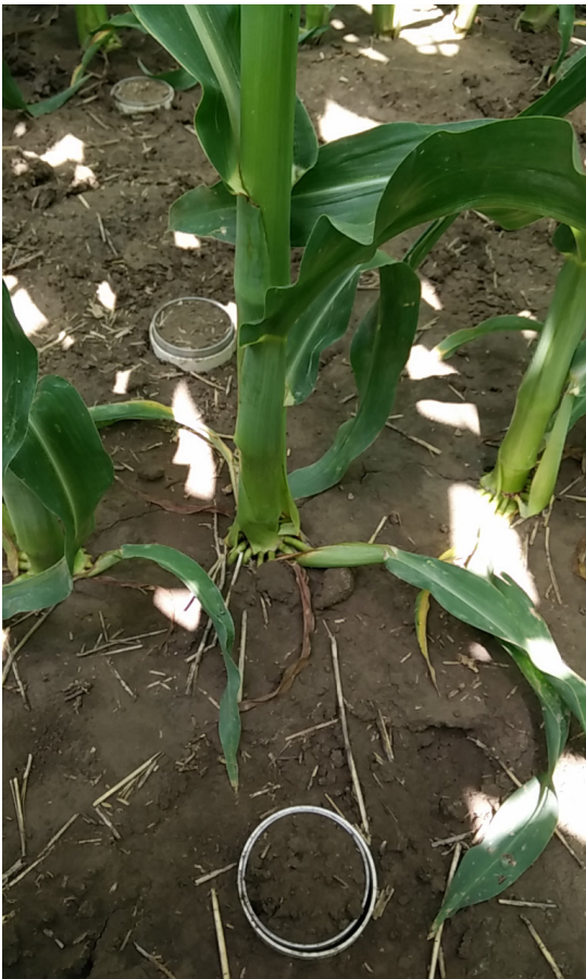
Figure 3. Measuring soil water evaporation using mini-lysimeter under spray nozzles and mobile drip irrigation at the Kansas State University Southwest Research-Extension Center, near Garden City, KS.
