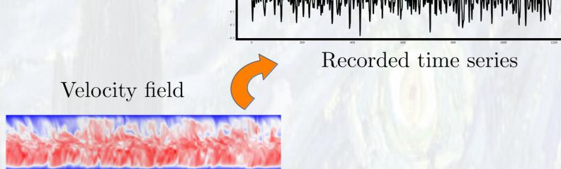
DNS of liquid metal flow in a channel with hot wall at the bottom (Paul Scherrer Institute, SUI)
