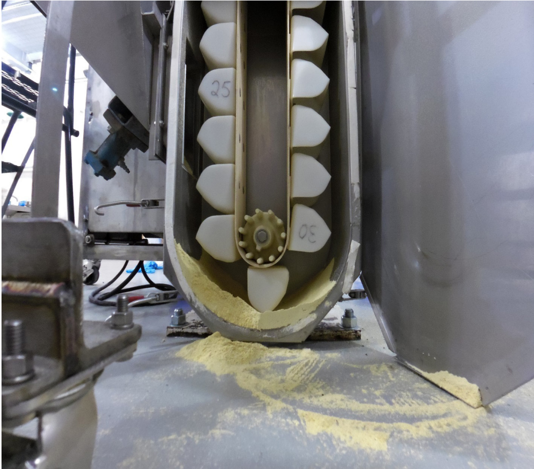
Figure 1. Charged boot from bucket elevator from this study demonstrates a potential area of cross-contamination. Sequences mimicked the subsequent feed manufactured in a commercial mill. Notably, the boot pit in this bucket elevator was shallow compared to that in most commercial systems, where the cross-contamination area can have a depth of multiple feet.
