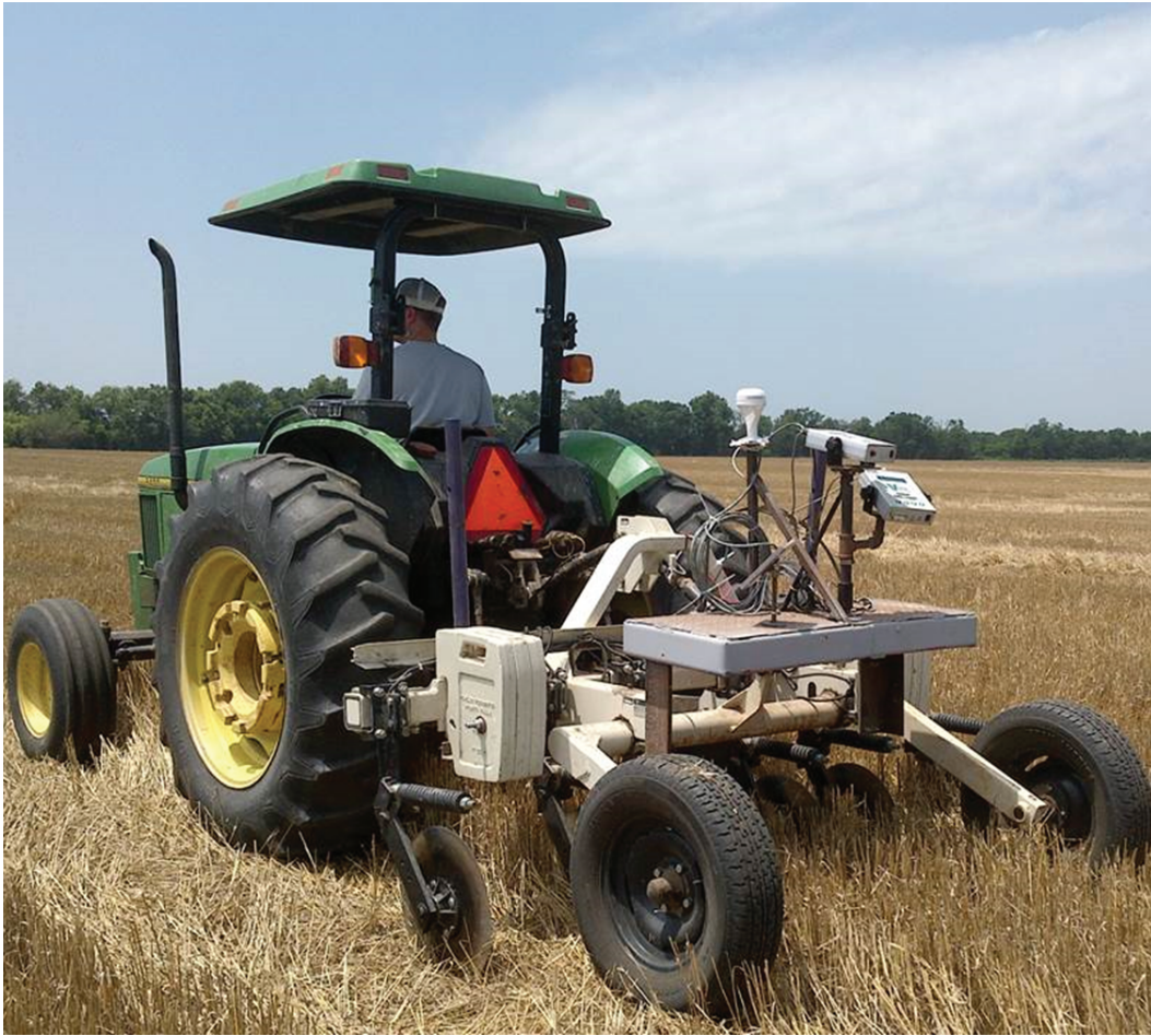
Figure 2. A Veris 3100 system was used to measure apparent soil electrical conductivity across the entire field.
