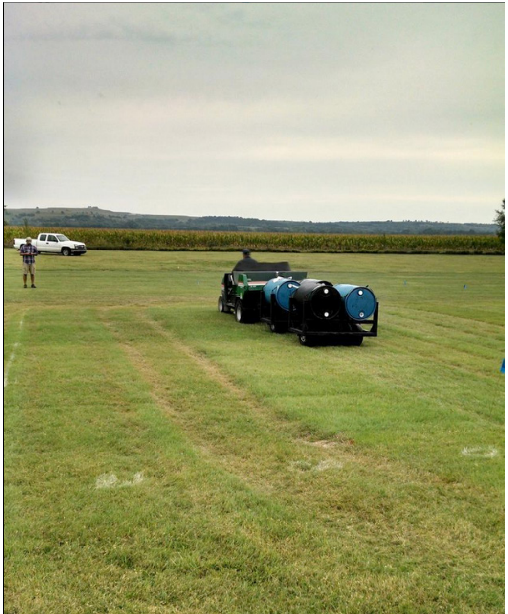
Figure 1. The golf cart traffic simulator used in this study consisted of two independent trailers with a solid axle. Simulator obtained equivalent lbs/in 2 tire weight of average golf cart with two golfers and clubs.
