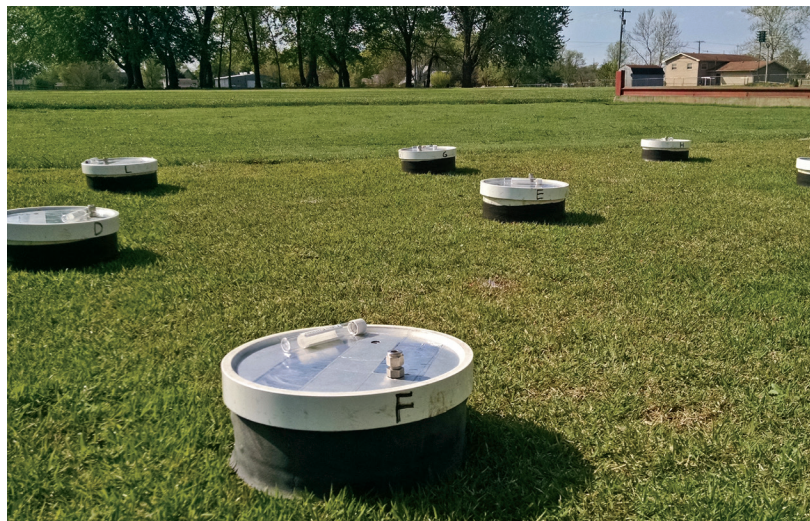
Figure 3. Close-up of one of twelve static chambers and vials used for sampling N 2 O.
