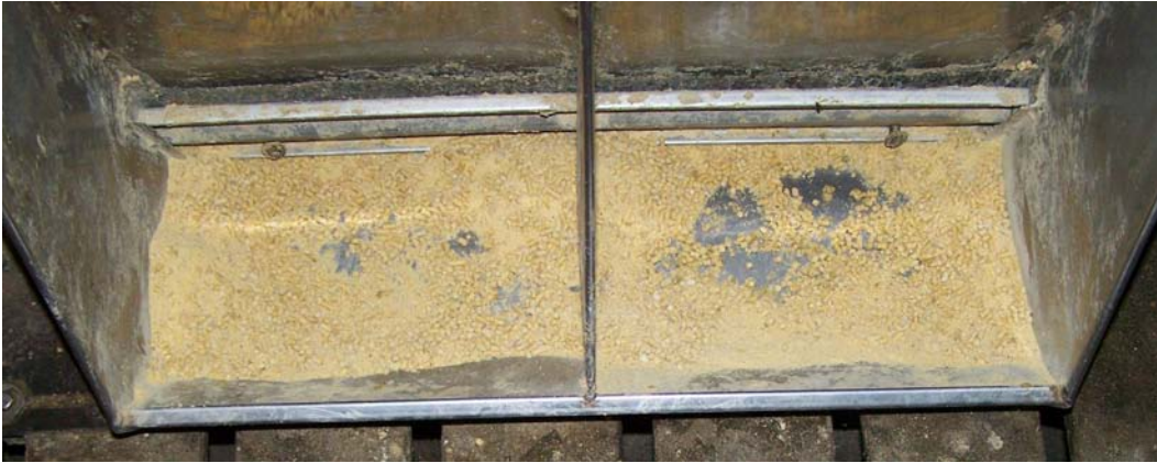
Figure 14. Phase 3 narrow feeder adjustment with 50% pellets and 50% fines (minimum feeder gap was 0.5 in. with a maximum gap of 0.75 in.) averaged 93% feeder pan coverage.
