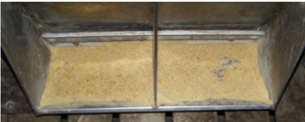
Figure 18. Phase 3 wide feeder adjustment with screened pellets (minimum feeder gap was 1.00 in. with a maximum gap of 1.25 in.) averaged 96% feeder pan coverage.
