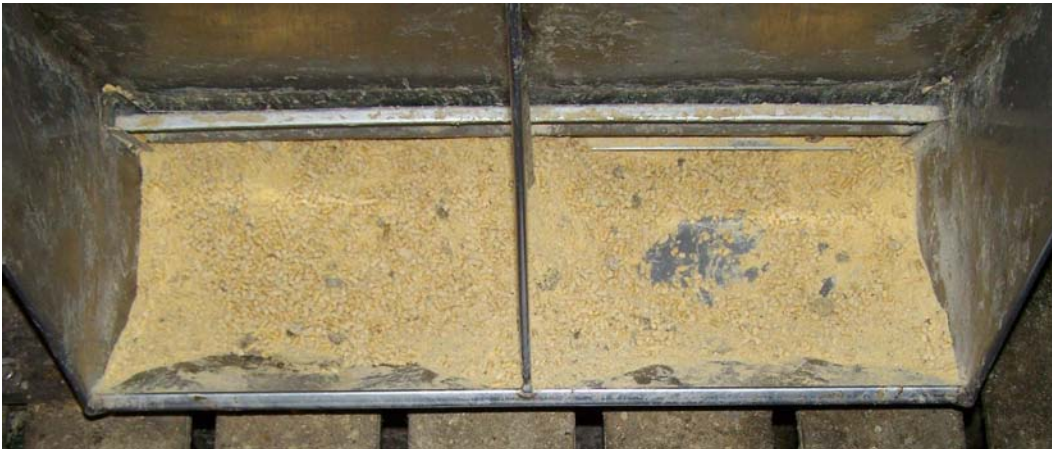
Figure 15. Phase 3 narrow feeder adjustment with screened pellets (minimum feeder gap was 0.5 in. with a maximum gap of 0.75 in.) averaged 92% feeder pan coverage.
