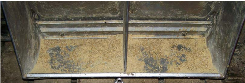
Figure 6. Phase 1 wide feeder adjustment with screened pellets (minimum feeder gap was 1.00 in. with a maximum gap of 1.25 in.) averaged 86% feeder pan coverage.
