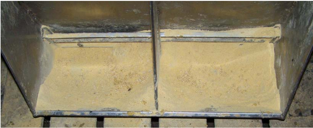
Figure 17. Phase 3 wide feeder adjustment with 50% pellets and 50% fines (minimum feeder gap was 1.00 in. with a maximum gap of 1.25 in.) averaged 99% feeder pan coverage.
