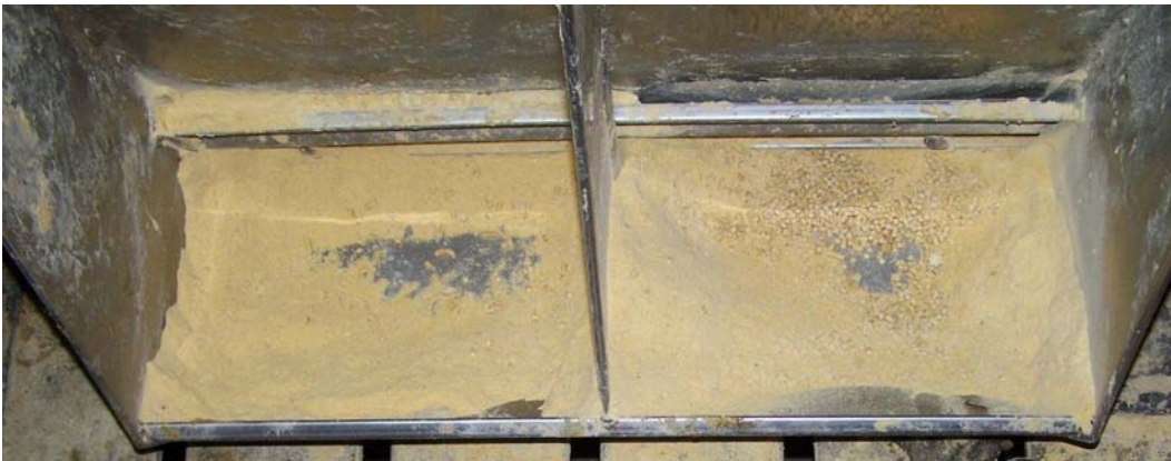
Figure 11. Phase 2 wide feeder adjustment with 50% pellets and 50% fines (minimum feeder gap was 1.00 in. with a maximum gap of 1.25 in.) averaged 99% feeder pan coverage.
