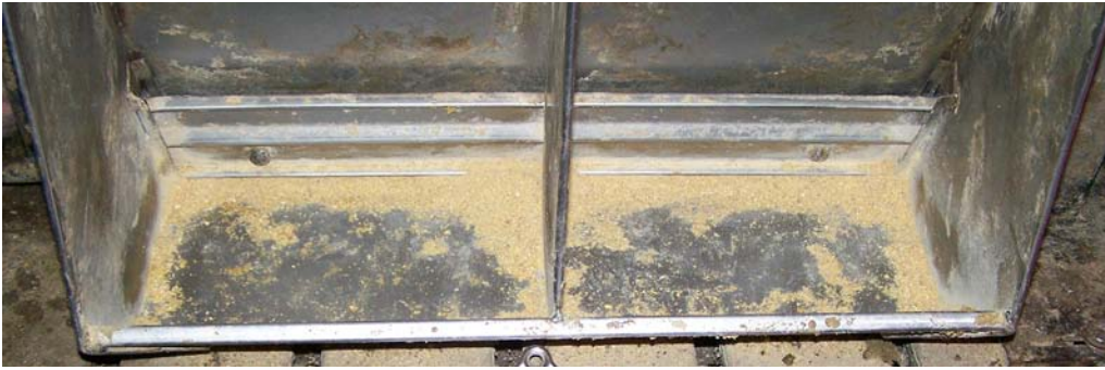
Figure 1. Phase 1 narrow feeder adjustment with meal diet (minimum feeder gap was 0.5 in. with a maximum gap of 0.75 in.) averaged 31% feeder pan coverage.
