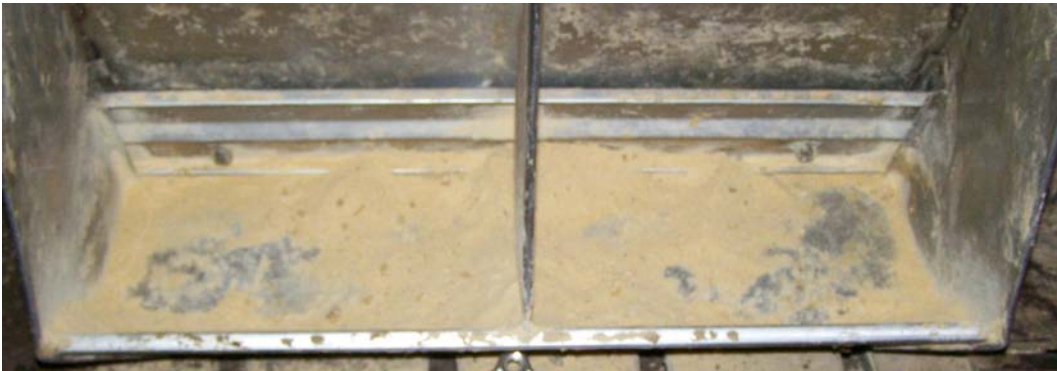
Figure 8. Phase 2 narrow feeder adjustment with 50% pellets and 50% fines (minimum feeder gap was 0.5 in. with a maximum gap of 0.75 in.) averaged 77% feeder pan coverage.
