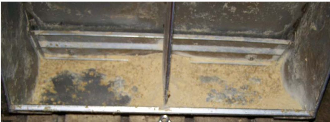
Figure 9. Phase 2 narrow feeder adjustment with screened pellets (minimum feeder gap was 0.5 in. with a maximum gap of 0.75 in.) averaged 69% feeder pan coverage.
