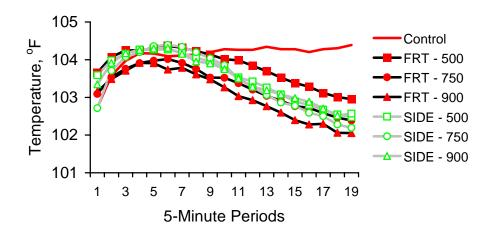
Control = no cooling system, FRT-500 = head to tail airflow at 500 CFM, FRT-750 = head to tail airflow at 750 CFM, FRT-900 = head to tail airflow at 900 CFM, SIDE-500 = right side airflow at 500 CFM, SIDE-750 = right side airflow at 750 CFM, and SIDE-900 = right side airflow at 900 CFM.
