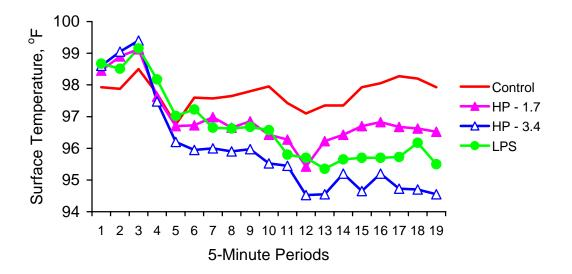
Control = no supplemental airflow or water treatment, HP-1.7 = 750 CFM airflow and 1.7 gallons/hour continuous high-pressure misting, HP-3.4 = 750 CFM airflow and 3.4 gallons/hour continuous high-pressure misting, and LPS = 750 CFM airflow and 4 gallons/hour of water via a low-pressure soaking system.
