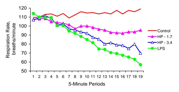
Control = no supplemental airflow or water treatment, HP-1.7 = 750 CFM airflow and 1.7 gallons/hour continuous high-pressure misting, HP-3.4 = 750 CFM airflow and 3.4 gallons/hour continuous high-pressure misting, and LPS = 750 CFM airflow and 4 gallons/hour of water via a low-pressure soaking system.
