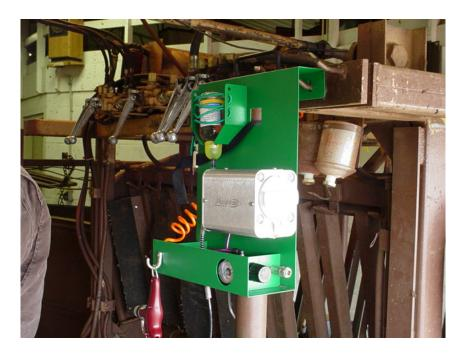
Figure 1. Felton Pulse 250 Needle-free Injection System.
