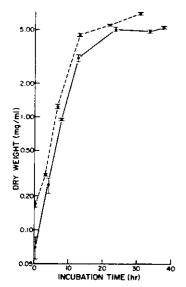
All of the cells from a growth flask were collected with the filtration device and washed on the filter with distilled water. Cells, filter paper and crucible were dried in on oven overnight at 90°C, cooled to room temperature, and weighed with a Mettler H-16 balance to within • 0. 1 mg. Net cell dry weight was calculated as the difference between gross and tare weights.
