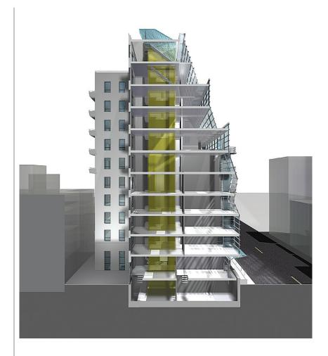
allows for the addition of a four-story penthouse in glass and steel. The setback intervals create a rooftop landscape which allow the outside in with large reflecting glass windows in a mediated transition.
