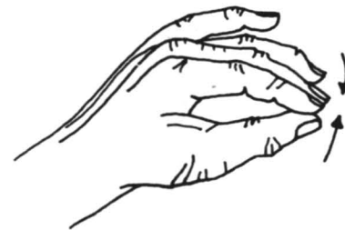
PALMAR PINCHING USES PADS OF THUMB, INDEX FINGER AND USUALLY THE MIDDLE FINGER
