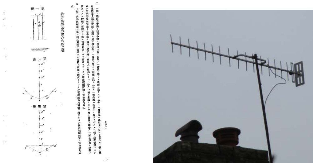
Figure 6. Shintaro Uda's publication of what came to be known as the Yagi-Uda antenna (left, 1926): the most common domestic television antenna (right).
