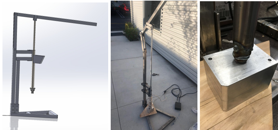
Figure 12: First iteration modeled injector design, final injector, and zoom in of reducer and mold
