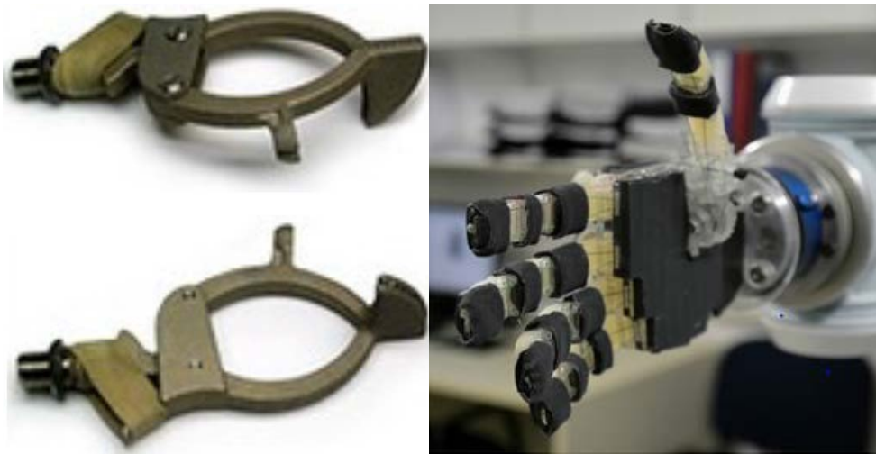
Figure 9: The Trautman Hook (left) and the OpenBionics (right) both were made from 3D printing so that people can have easier accessibility to upper limb prosthetics (Phillips et al. 2015).
