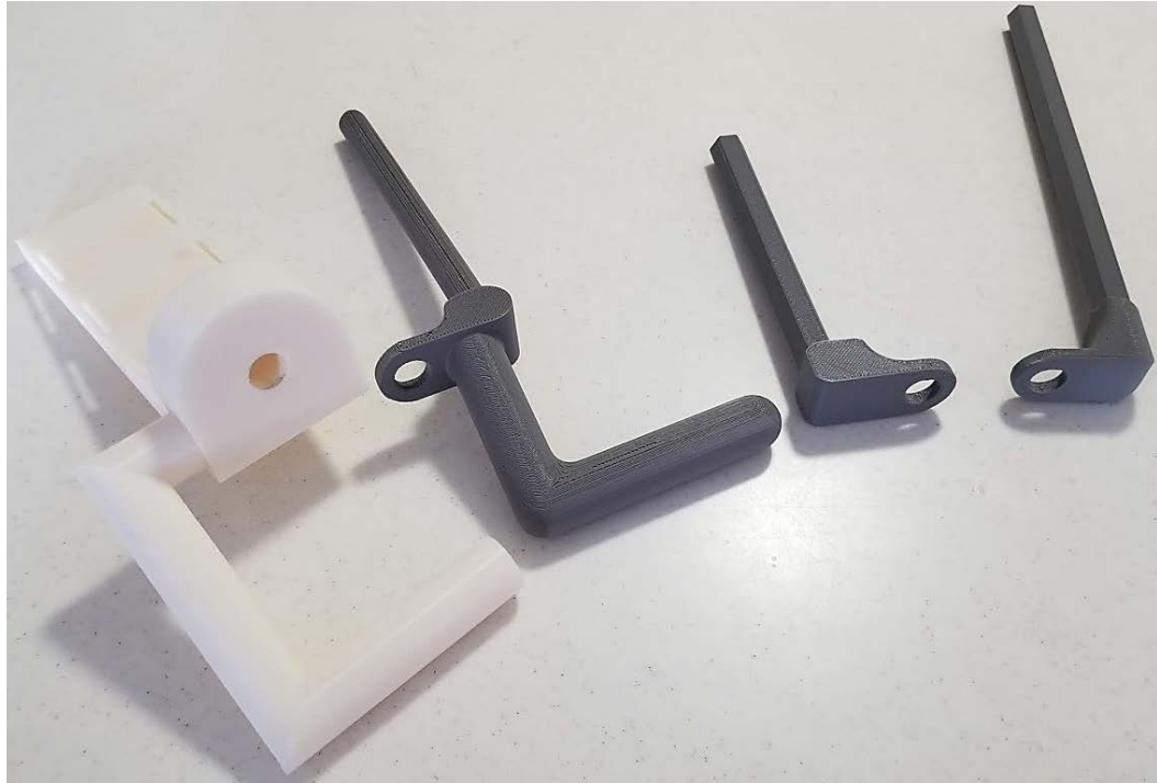
Figure 27: The prosthetic simulator iterations. The first being on the left, and the final above-arm and below-arm simulators on the right. The second iteration is the part second from the left.
