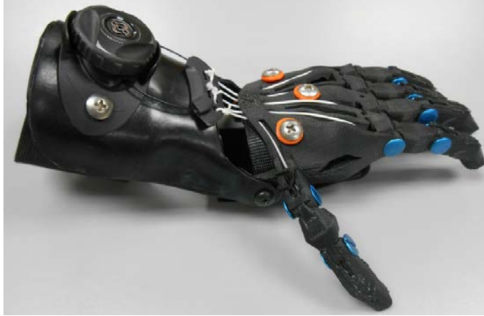
Figure 8: Cyborg Beast 3D printable prosthetic hand. A low-costing upper limb prosthetic design to fit children.
