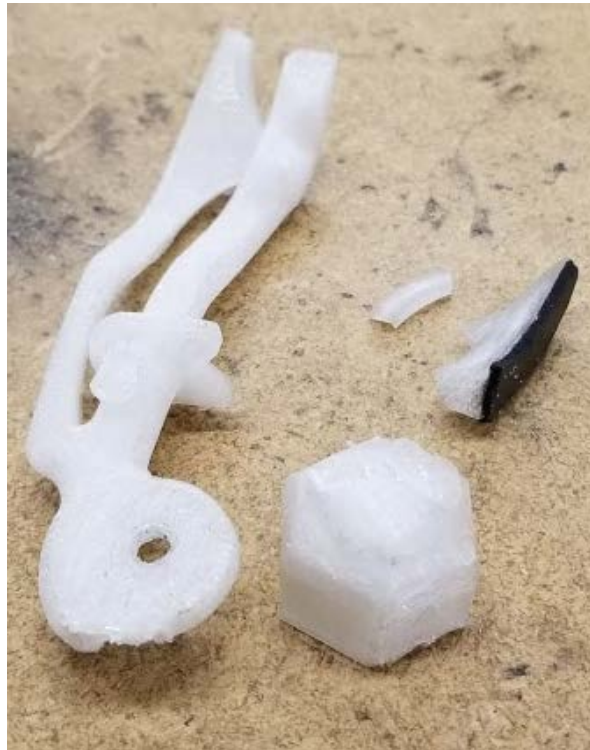
Figure 42: Post stress test of screw-housing half of the 3D printed prosthetic with truss.
