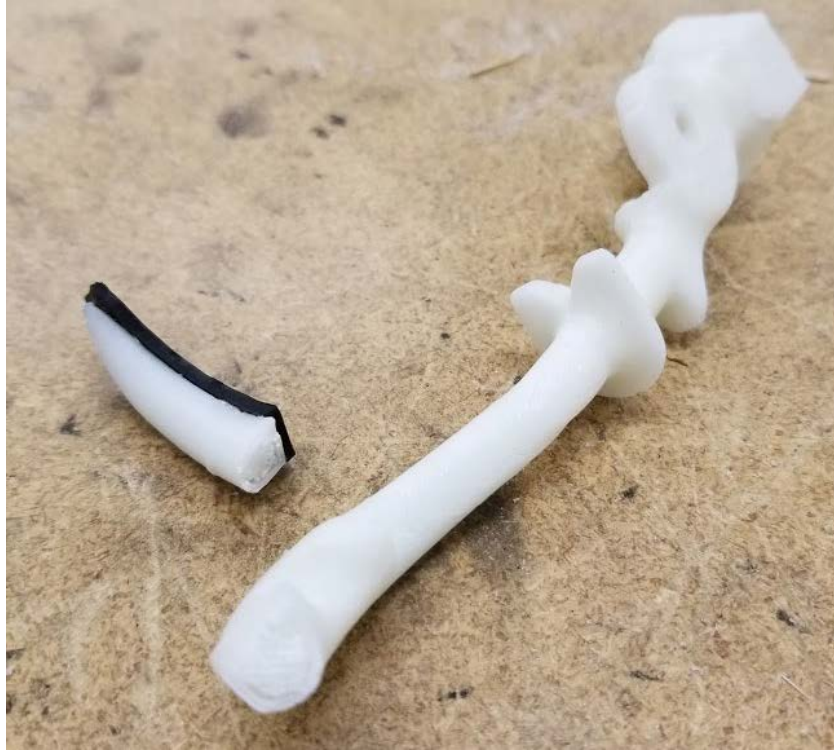
Figure 41: Post stress test of screw-housing half of the 3D printed prosthetic with no truss.
