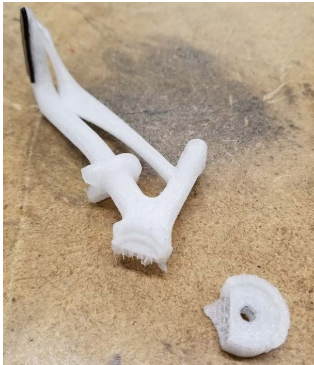
Figure 44: Post stress test of thumb half of the 3D printed prosthetic with truss.
