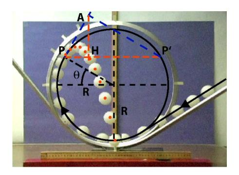
Fig. 2. Results of our demonstration for  $\theta=30^\circ$ . Video editing software was used to produce a "stroboscopic" picture of the motion. The position of the center-of-mass of the falling ball is indicated by the red dots. The geometrical construction is similar to the one in Fig. 1.
