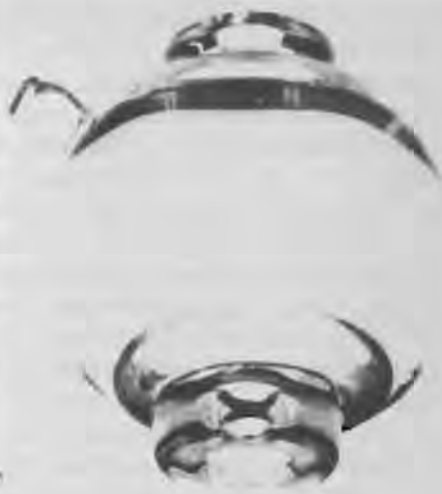
FIG. 6. Labeled release Pyrex glass nutrient ampoule showing the fill port extending to the lower right and the two collars surrounding the puncture discs.
