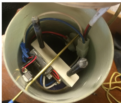
Figure 13. Inside View of the Avionics Bay
