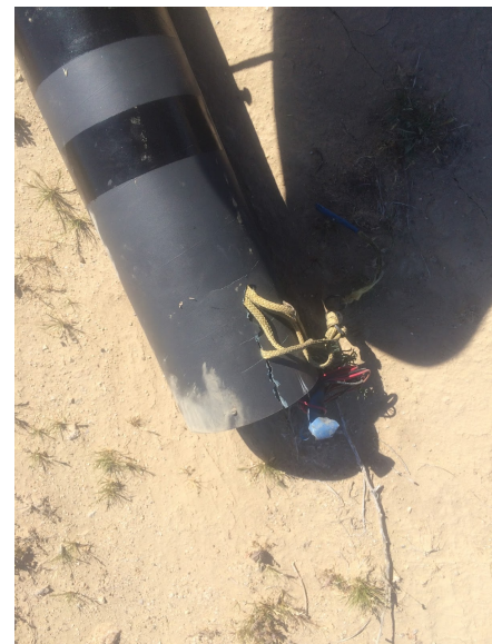
Figure 27: Zippering on Main Deployment
