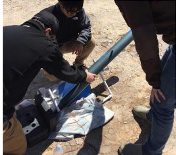
Figure 23. Setup for the drogue black powder charge test Figure 24. Setup for the main black powder charge test
